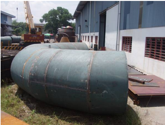
Elbow and ducting
